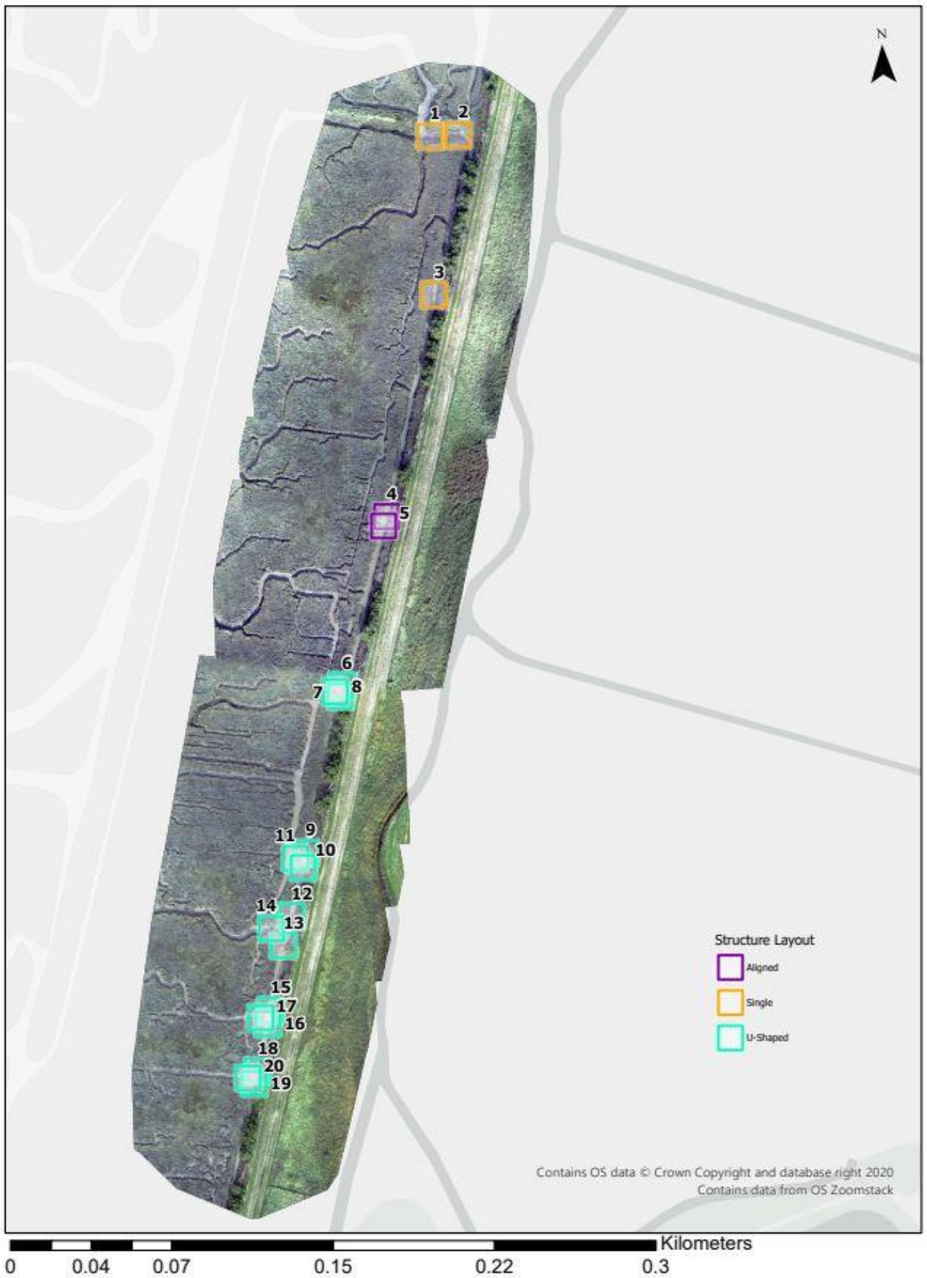
Figure 2 Moverons Farm coir roll structure locations with associated structure layout.
