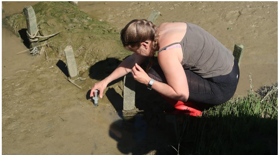
Figure 12 Taking a sediment core from one of the coir roll structures
